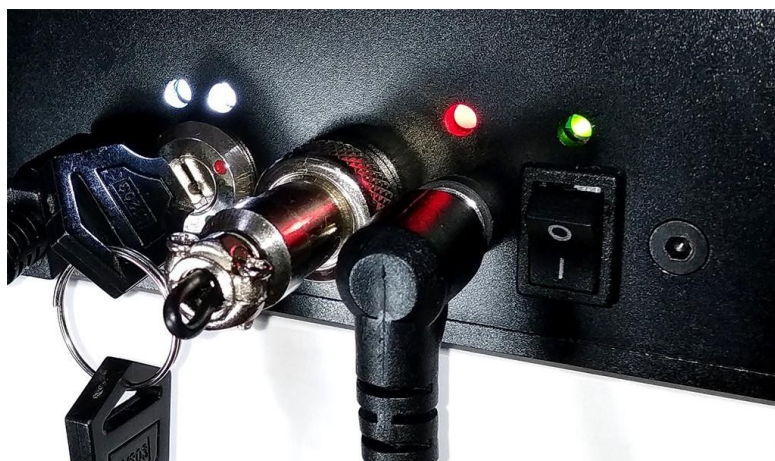
Safety key, power input, LEDs, and power switch example
