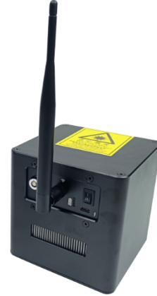
A11 rear side with antenna
