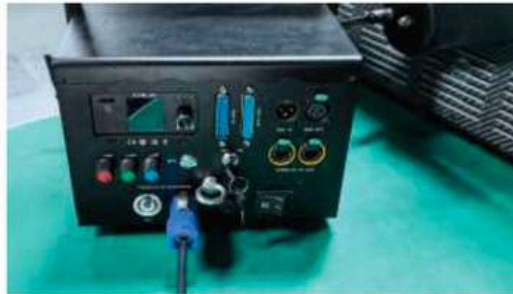
A: Use the supplied Neutrik powercon cable to connect the laser projector to a AC main power supply by using the input connector. Insert the safety keys(remain in the Off position).
