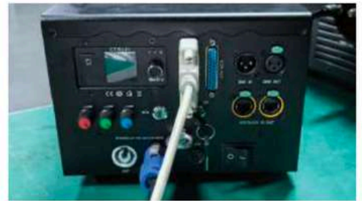
B: To control the system by using an external signal e.g. ILDA or Ethernet(if FB4 built-in), plug the corresponding cable to the input connector at the back of the laser system.
