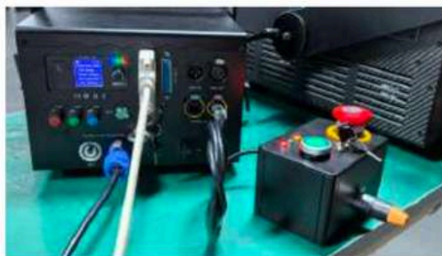
G: After the emission delay period of about 10-14s, the laser system is ready to start output laser emission by Enabling output thru laser software. (Over these steps, the laser system is controlled by ILDA signal, in which way, make sure that the ILDA cable is well connected between the projector and the ILDA DAC controller which has to be well connected to the PC as well).
