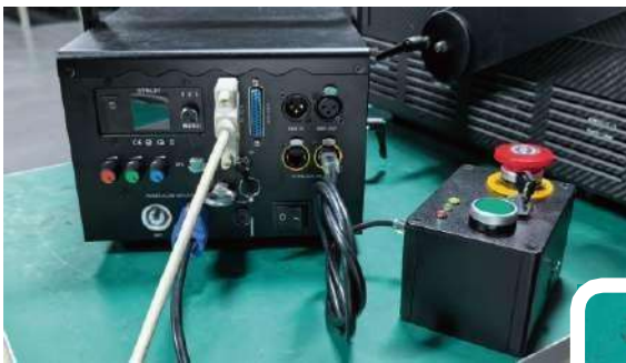
C: Connect the E-stop box to the socket marked as INTERLOCK IN with a supplied CAT5/6 cable.
