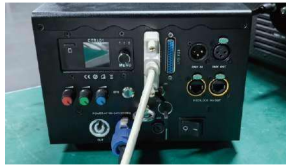
B: To control the system by using an external signal e.g. ILDA or Ethernet(if FB4 built-in), plug the corresponding cable to the input connector at the back of the laser system.
