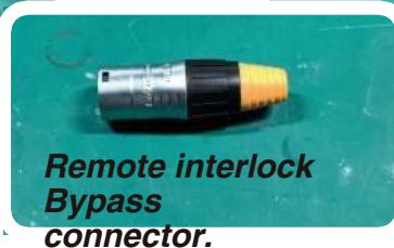
D: Insert the Remote interlock Bypass connector to the E-stop box and turn the key to on to disable the INTERLOCK (the US regulations).
