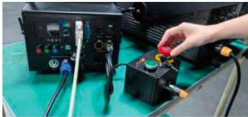
E: Release the E-stop button by anti-clockwise rotation, and the button will be pulled upwards.
