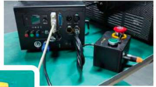
D: Insert the Remote interlock Bypass connector to the E-stop box and turn the key to on to disable the INTERLOCK (the US regulations).
