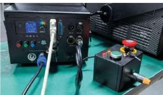
G: After the emission delay period of about 10-14s, the laser system is ready to start output laser emission by Enabling output thru laser software.
