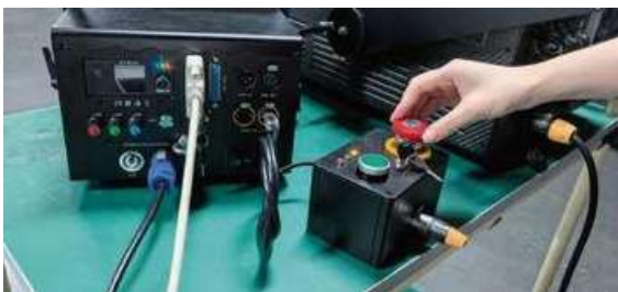
E: Release the E-stop button by clockwise rotation, and the button will be pulled upwards.
