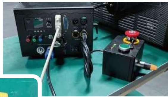
D: Insert the Remote interlock Bypass connector to the E-stop box and turn the key to on to disable the INTERLOCK (the US regulations).
