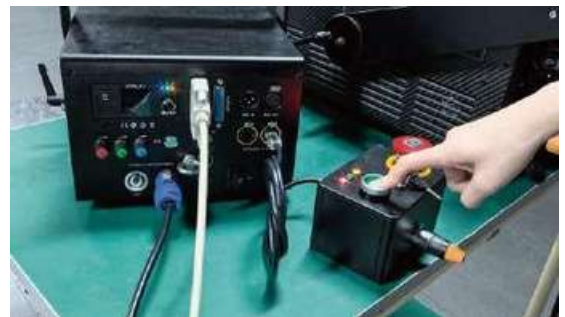
F: Press down the START button on the E-stop box. Turn the keys and the power switch at the back of the laser system to the ON positions.
